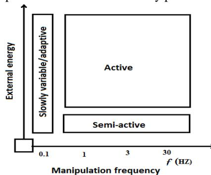
Fig. 2: Comparison between passive, adaptive, semi-active system.
