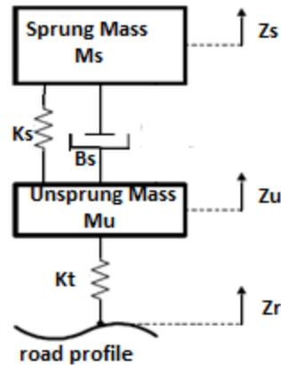
Figure1. b: Block Diagram of Passive Suspension System of quarter car model
