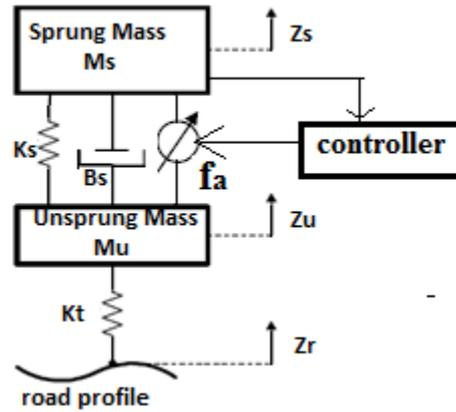
Fig.3: Suspension system block diagram
